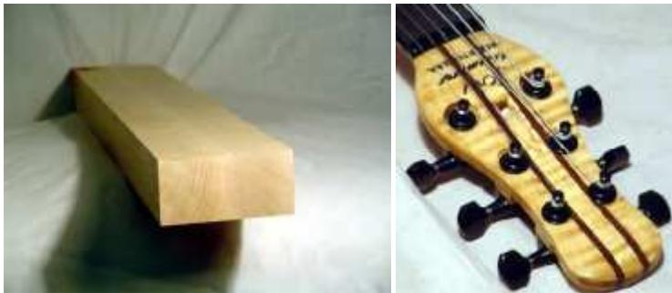
A flat-sawn neck is the most common especially in electric guitars. They have a lower string tension than an acoustic, and with a truss rod, a flat sawn neck is usually sufficient, however, it is more prone to bowing up or down. Flat-sawing wood gets the most yield out of a log, and therefore is a cheaper, more economical wood. All you have to do is cut the board down into a neck blank and start shaping.
